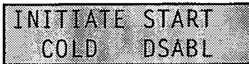
Figure 3-31. Setup Screen 19 - INitiate GPS START
